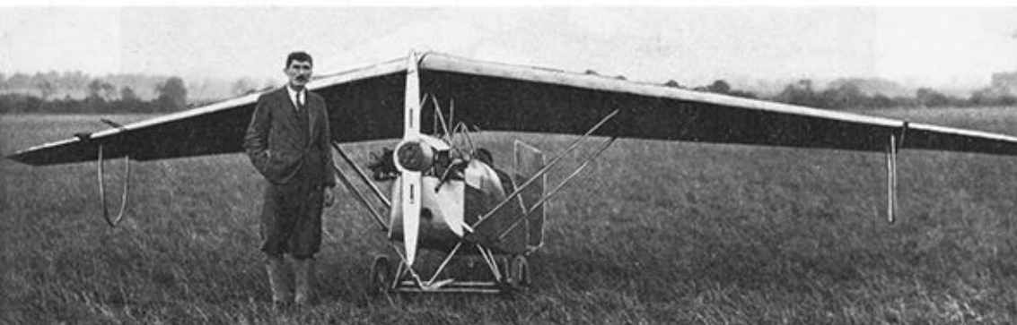
This tail-less aircraft, pictured in 1930, was built by two Nottingham men over a period of four years. On its first flight it covered several miles and reached a height of 1,000ft. Pictured with it is Mr. R. F. T. Granger, the designer.
