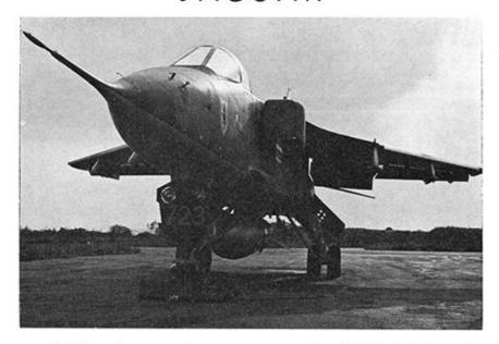
Making its second appearance at the SSAFA Display, the Anglo-French Jaguar tactical support and training aircraft first flew in 1968. A joint production of the British Aircraft Corporation and Avions Marcel Dassault/Breguet Aviation companies, it is powered by two Rolls-Royce Turbomeca Adour turbofan engines with afterburners.
