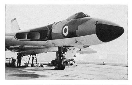
The Vulcan B.2 can fly at very high level or beneath enemy radar at very low level. Developed from the B.1, the world's first large delta-wing bomber, its configuration gives a unique combination of load-carrying capabilities, high subsonic speed and long range. It is powered by four 20,000lb. thrust Bristol-Siddeley Olympus turbojets and can be refuelled in flight. Span: 111ft.; length 99ft. 11ins.; height 27ft. 2ins.
