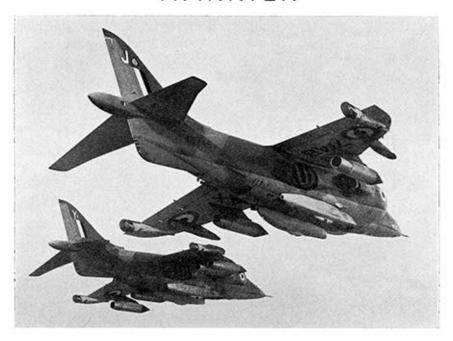
The Harrier was the world's first operational V/STOL ground attack fighter. It can take off and land vertically and even fly sideways and backwards. It is particularly valuable in close support—operating from small, unprepared strips otherwise practicable for helicopters only. This is the first time a Harrier has appeared in the SSAFA Display. Span 22ft. 10ins.; length 42ft.; height 10ft.
